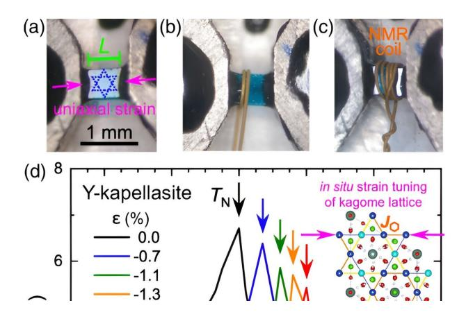
In situ strain tuning of frustrated magnetism in  $Y_3Cu_9(OH)_{19}Cl_8$ . (a)–(c) For NMR experiments under uniaxial strain a single crystal was glued between the two arms of a piezoelectric strain cell (a), and, subsequently, an NMR coil was wound around it (b),(c). (d)  $T_1^{-1}$  was measured for B || a upon uniaxial compression of the kagome lattice parallel to the Cu<sup>2+</sup> chains. Credit: *Physical Review Letters* (2023). DOI: 10.1103/PhysRevLett.131.256501
