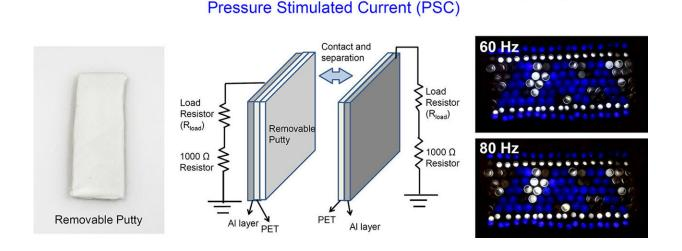
Novel Contact-Separation Generator Using Limestone Mounting Putty via
