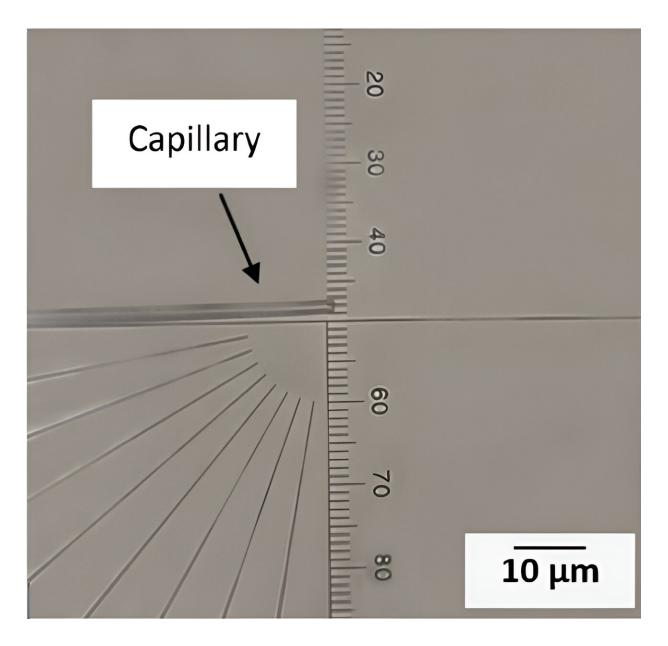
View of the capillary in the microforge. The left side of the picture shows the capillary. The distance between each mark on the scale is 3 µm. Credit: *Scientific Reports*, doi: 10.1038/s41598-023-49128-8
