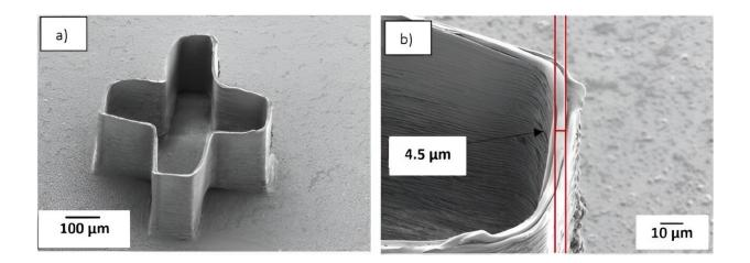
(a) The SEM image of 3D printed cross-shaped structure with more than 300 layers. (b) The width of the fiber of the top layer is 4.5  $\mu$ m. The structure printed with long taper 3–9 capillary and ink with 10% (50 kDa). Credit: *Scientific Reports*, doi: 10.1038/s41598-023-49128-8
