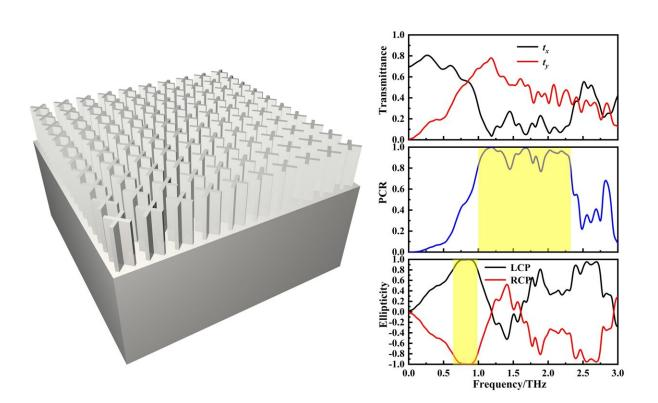
Schematic diagram of the structure and polarization conversion effects. Credit: *Frontiers of Optoelectronics* (2023). DOI: 10.1007/s12200-023-00098-9
