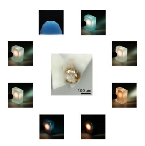
Tellurite glasses containing a  $\sim 200 \ \mu m$  gold particle (middle photo) and gold nanoparticles of different size and quantity (surrounding photos). Credit: Laurence Deziel
