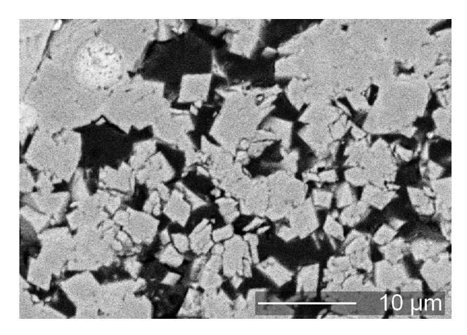
Scanning electron microscope image using material taken in the drill core from the borehole taken in 1981 from the Nördlinger Ries reveals dolomite crystals with rhombohedral shape. Credit: Lingqi Zeng, Göttingen University
