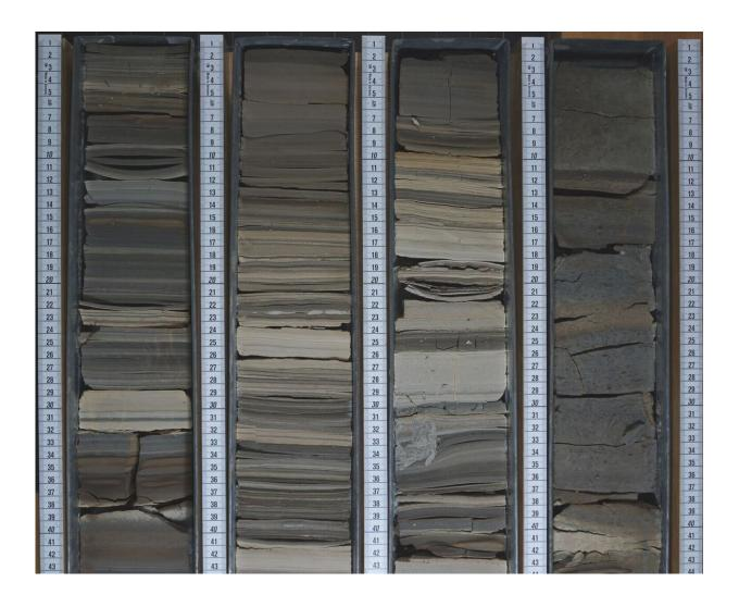
Drill core from borehole taken in 1981 from the Nördlinger Ries. There are distinctive layers of light-colored dolomite between fine-layered dark sediments of the former crater lake. Credit: Gernot Arp, Göttingen University
