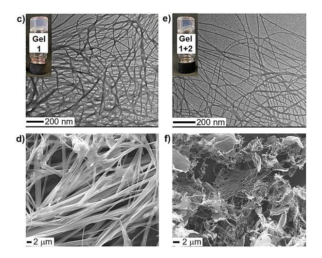
Images from two different electron microscopy analyses of Fmoc-pentafluorophenylalanine hydrogel alone (c-d) and with a partner molecule (e-f). Inset: photos of the two hydrogels. Credit: Politecnico di Milano
