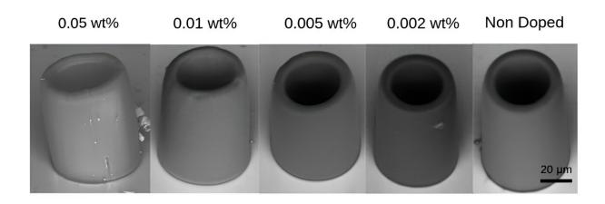
Cylindrical microstructures formed by a photoresist doped with different proportions of nanodiamond are shown in these scanning electron microscope images. Credit: IFSC-USP
