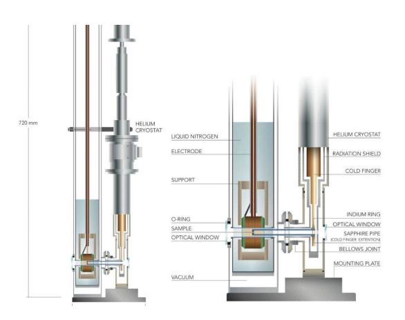
A graphic illustrates the setup and functions for the Rice Advanced Magnet with Broadband Optics, or RAMBO, a unique instrument that lets researchers use pulsed-laser spectroscopy to examine the behavior of materials that are simultaneously cooled near absolute zero and subjected to a massive pulse of magnetic energy. Credit: Junichiro Kono Laboratory
