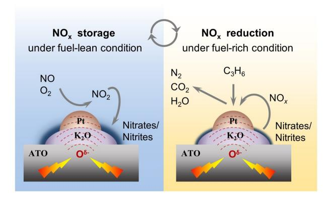
The procedure of electrified NOx storage-reduction. Credit: NIMTE
