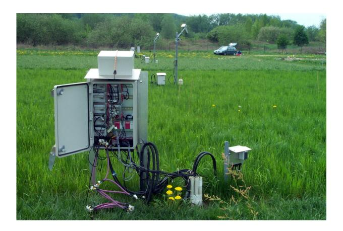
Internal view of the cable data logger box for the soil temperature measurement system (Controller Area Network bus module system) at the Jena experimental site. Credit: Karl Kübler / MPI BGC Jena
