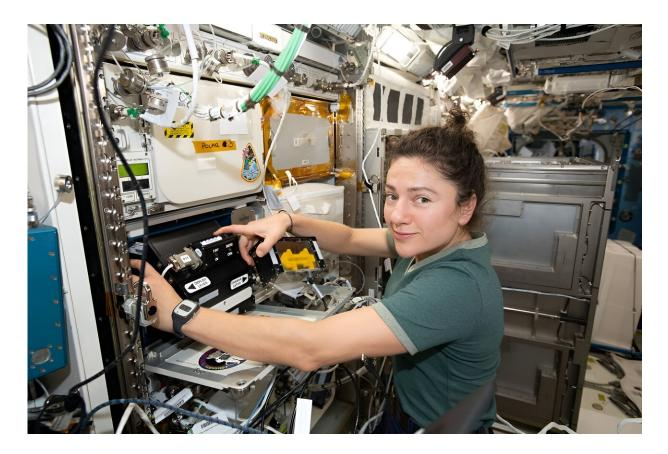
NASA astronaut Jessica Meir installs the Bone Densitometer device for the Rodent Research 19 experiment. Credit: NASA
