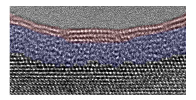
A transmission electron microscopy image of the oxidized aluminum surface shows that the passivating oxide film formed in water vapor consists of an inner amorphous aluminum oxide layer and an outer crystalline aluminum hydroxide layer. Credit: Provided.
