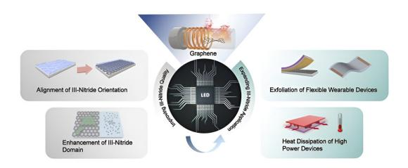
Application of transfer-free graphene on insulating substrates for III-nitride epitaxy. Credit: Science China Press
