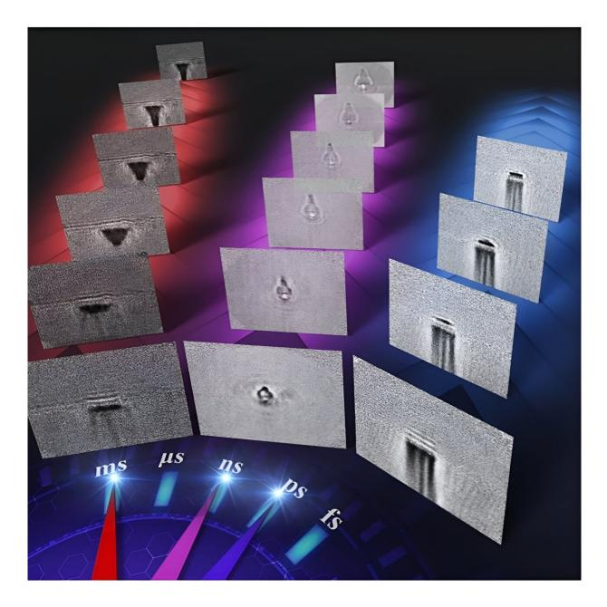
Images of laser ablation taken using the ultrawide time range, high-speed camera: Applying this new imaging technology, the researchers could see the propagating shock wave and plasma and the progress of laser processing over multi-timescales (about 10–100 picoseconds, about 1–10 nanoseconds, and about 1–100 milliseconds). Credit: 2023 Saiki et al./ CC BY NC
