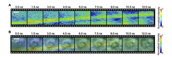
Observation of underwater shock wave through a biological cell. (A and B) STAMP movies with nine frames and an interval of 1.5 ns showing the propagation of underwater shock waves with (B) and without (A) a HeLa cell. Scale bars, 10 µm. Credit: *Science Advances* (2023). DOI: 10.1126/sciadv.adj8608
