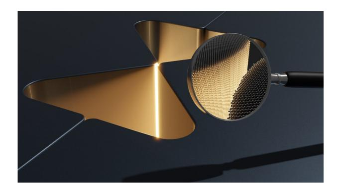
Illustration of the core of the photonic cavity that was fabricated as two halves that assembled themselves into one unit. The cavity confines light inside the gap, which is only a few atoms wide as indicated in the field of view of the magnifying glass. Illustration by Thor A. S. Weis. Credit: Thor A. S. Weis.
