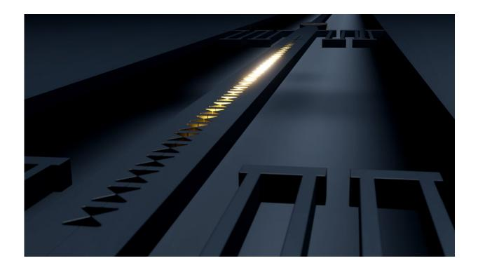
The self-assembled cavity can be integrated into larger self-assembled components for routing light around an optical chip. The figure shows the optical cavity embedded in a circuit containing multiple self-assembled elements. Illustration by Thor A. S. Weis. Credit: Thor A. S. Weis.
