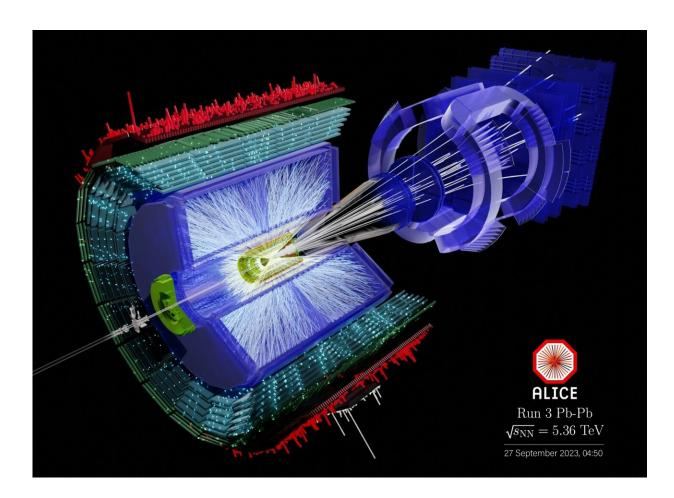
A lead-lead collision event in the ALICE detector. Credit: CERN
