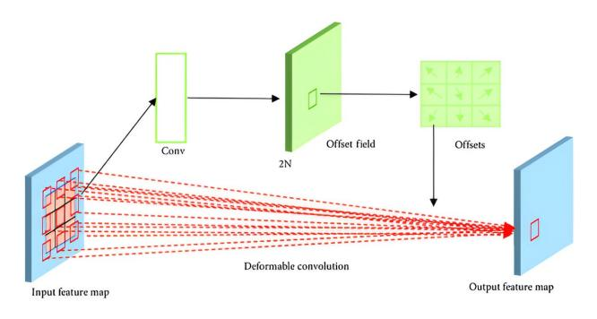
Architecture of a 3 × 3 deformable convolution. Credit: *Plant Phenomics* (2023). DOI: 10.34133/plantphenomics.0088
