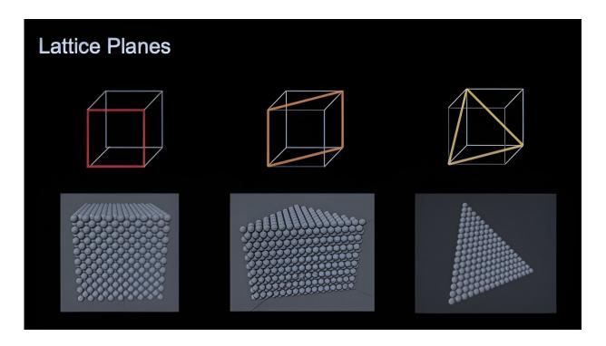
This image demonstrates how three families of planes in the face-centered cube extended crystal lattice are defined relative to the unit cell, how atoms are packed on the surfaces of these planes, and how these planes can form the crystal facets of three nanoparticle shapes. Credit: Anne Bentley / Lewis & Clark College
