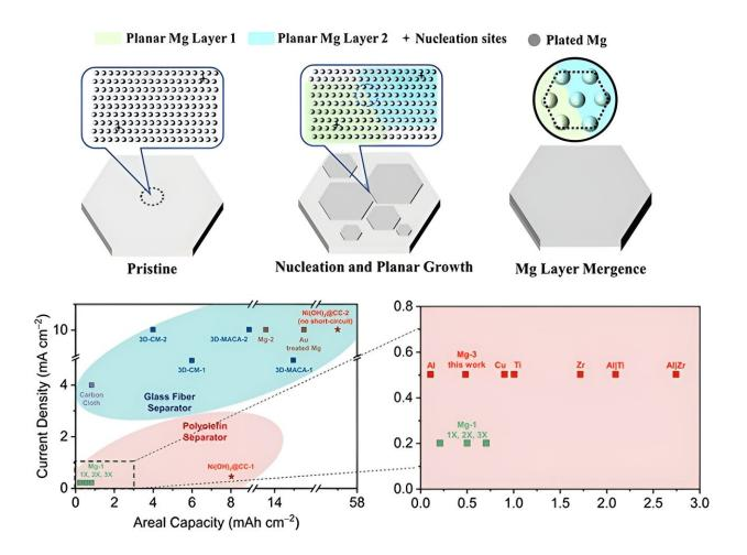
Schematic diagram of layer-by-layer planar growth model of Mg deposits and the performance comparison of various electroplating substrates. Credit: Wang Guixin & Du Aobing
