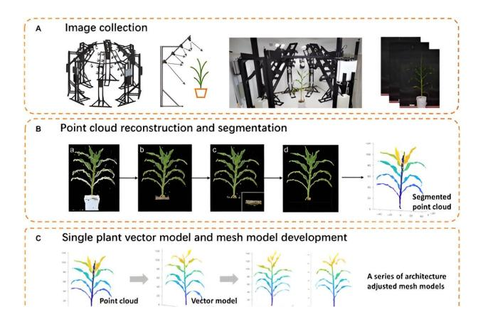
The pipeline of 3D canopy modeling. Credit: Plant Phenomics
