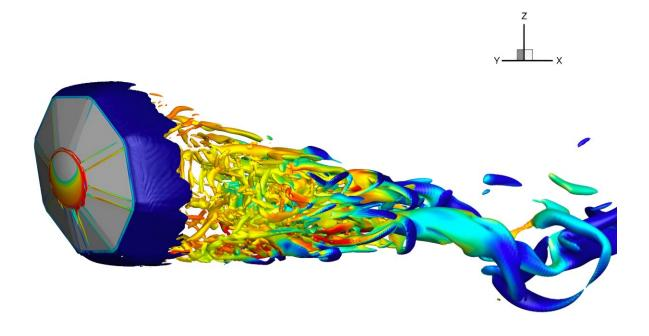
Free-flight simulation of the Adaptable Deployable Entry and Placement Technology vehicle showing Q-criterion, which is a measure of the amount of vorticity in the aerodynamic flow. The iso-contours indicate vortex structure, indicating lower vorticity in blue and higher vorticity in red. Credit: NASA/Joseph Brock
