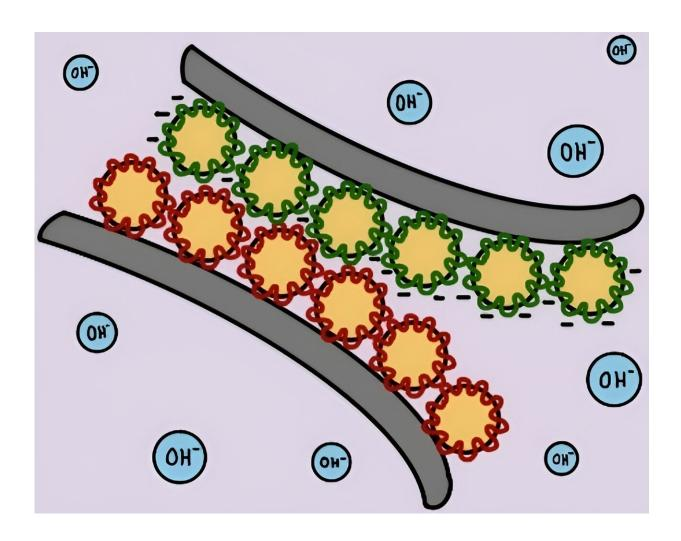
A reversible water-based electrostatic adhesive has been developed through conventional emulsion polymerization using commodity materials. It is made of two formulations, one containing a polycation, and other a polyanion. Detachment is only promoted in highly acidic or alkaline solutions as polyelectrolytes show distinctive charged states. This kind of adhesive would be
