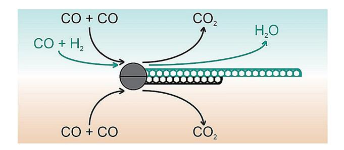
Schematic representation of hydrogen's effect in CO-based CVD synthesis of nanotubes. Credit: Ilya Novikov et al./*Chemical Engineering Journal*
