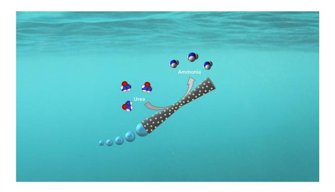
The outside of the micromotor in this study is coated with the chemical compound laccase. This enables the motor to convert the urea in the water into ammonia. Credit: Institute of Chemical Research of Catalonia (ICIQ)
