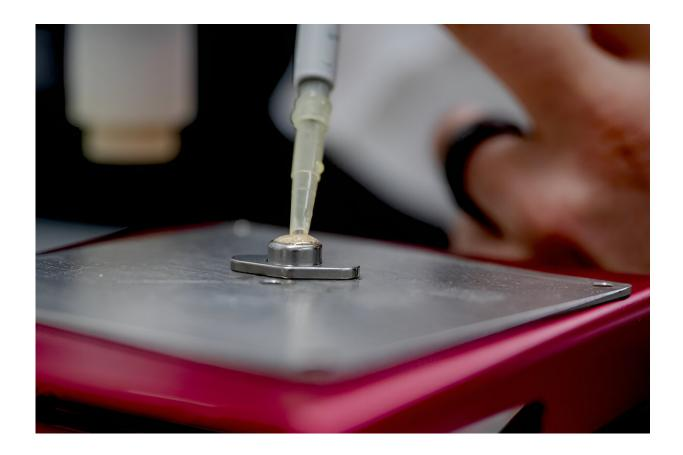
The sample consisting of the beads (with enzymes bound to them) and buffer is placed on a small metal plate to ensure good conductivity during the subsequent plasma treatment. Credit: RUB, Marquard
