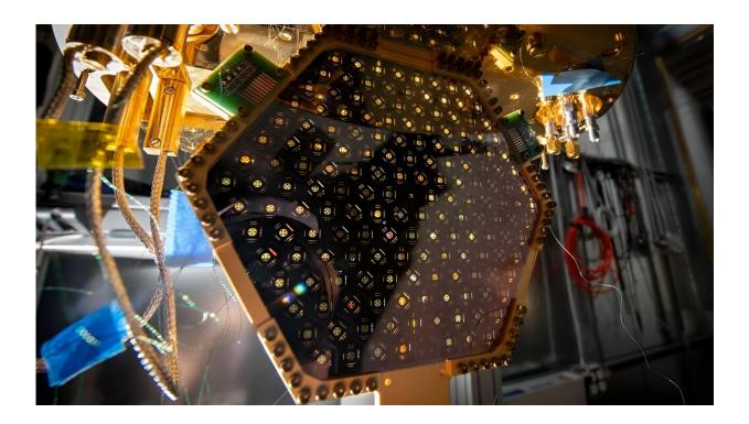
A photograph of a CMB-S4 detector wafer being prepared for testing in a cryostat at Lawrence Berkeley National Laboratory. Credit: Thor Swift/Lawrence Berkeley National Laboratory
