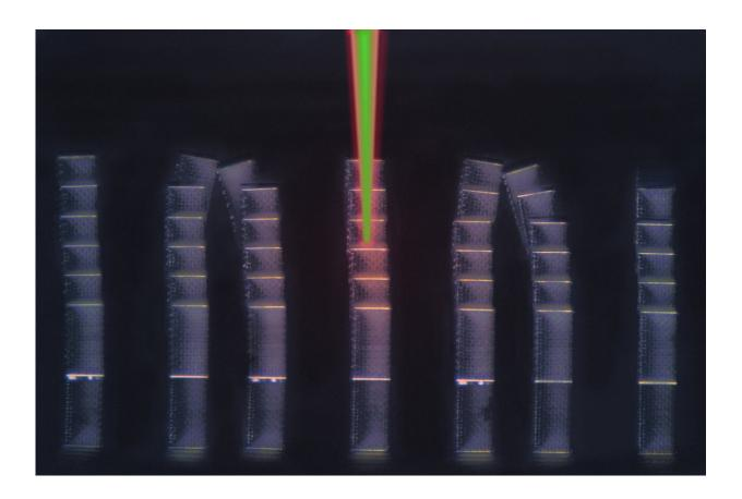
This optical micrograph shows an array of microscopic metamaterial samples on a reflective substrate. Laser pulses have been digitally added, depicting pump (red) and probe (green) pulses diagnosing a sample in the center. The LIRAS technique sweeps through all samples on the substrate within minutes. Credit: Carlos Portela, Yun Kai, et al
