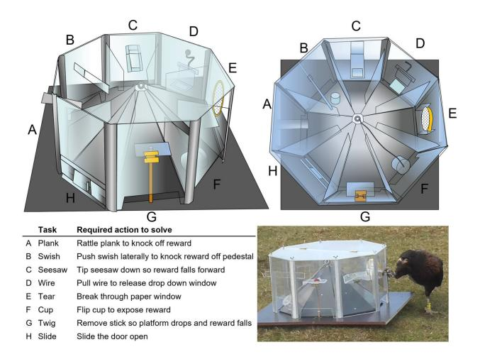
Eight-task innovation box and movements required to solve each task panel. Octagonal transparent Perspex innovation box with a transparent lid, eight removable transparent Perspex task panels (17 × 24 cm), and an opaque wooden base, custom-built by Markus Fitzka (Messerli Research Institute, University of Veterinary Medicine, Vienna). Bottom left: movement required to solve each task panel. Bottom right: a juvenile striated caracara uses a foot to solve the
