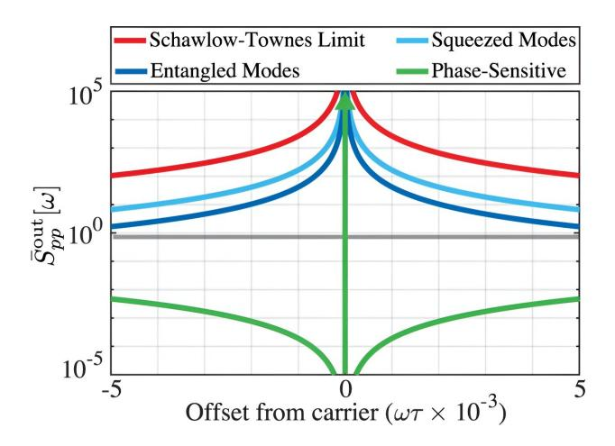
Phase noise of quantum-enhanced feedback oscillators. Spectra of the output phase quadrature for four types of quantum noise-limited oscillators. Red shows the Schawlow-Townes spectrum of an oscillator with phase-insensitive amplifier and the in-coupled and ancillary modes in vacuum. Light and darker blues depict the case where these modes are squeezed (light blue) and entangled (dark blue)
