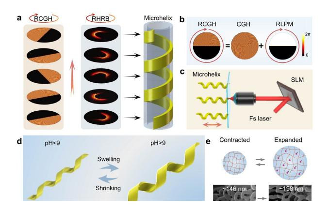
Schematic illustration of highly efficient fabrication of stimuli-responsive microhelix based on the rotary holographic processing method. Credit: *Light: Advanced Manufacturing* (2023). DOI: 10.37188/lam.2023.029
