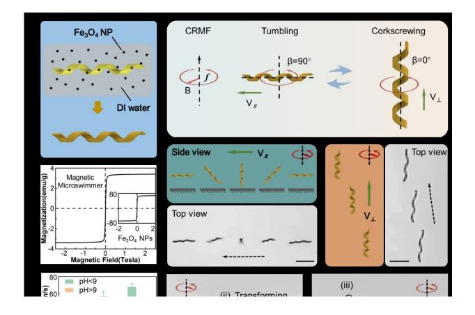
The adaptive locomotion of shape-morphing helical microswimmer. Credit: *Light: Advanced Manufacturing* (2023). DOI: 10.37188/lam.2023.029
