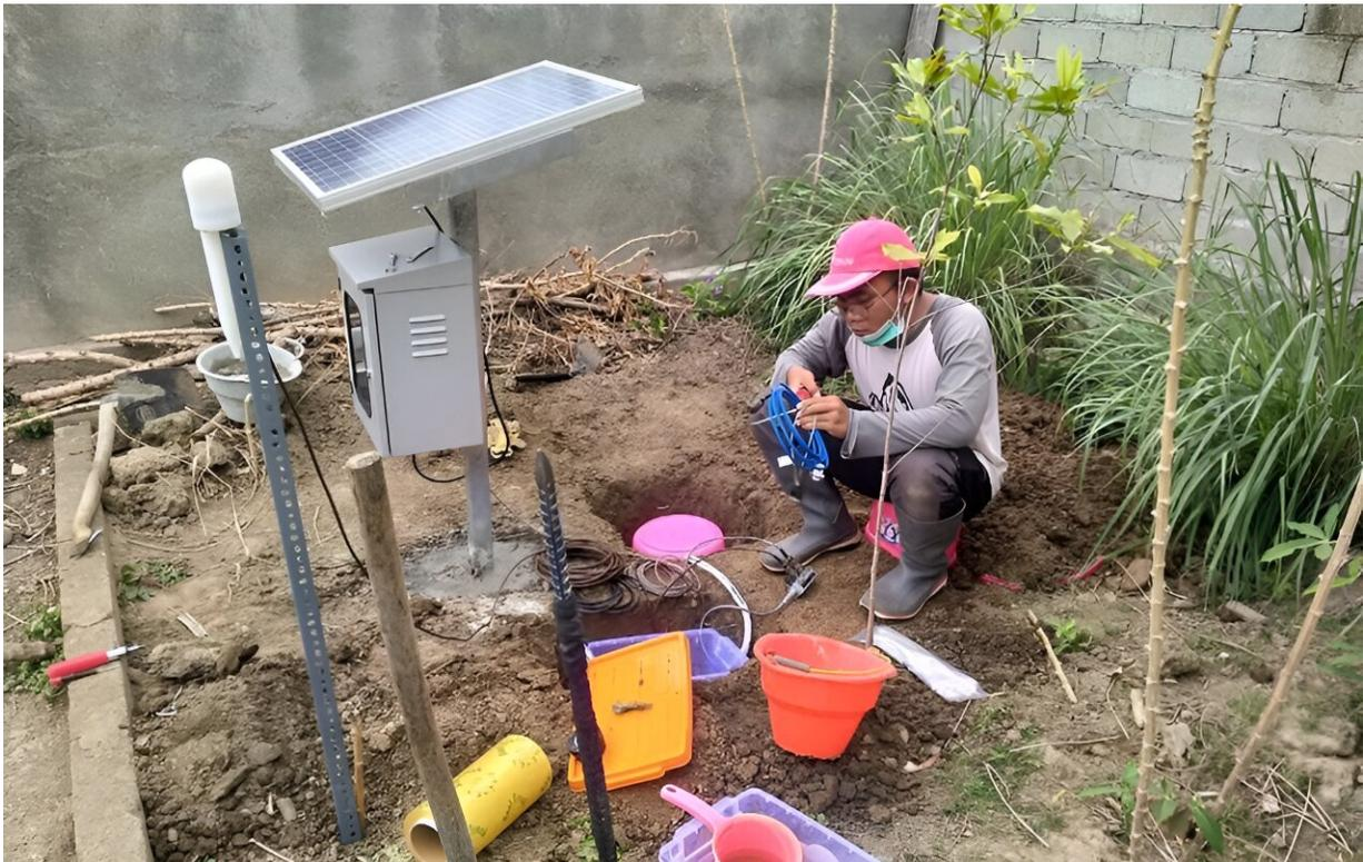
Researcher from the Institut Teknologi Bandung in Indonesia installs one of the seismic stations close to the proposed site of the new capita. Credit: ITB
