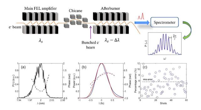
Schematic layout of the proposed method and spectrotemporal reconstructions of attosecond X-ray free-electron laser pulses. Credit: SARI
