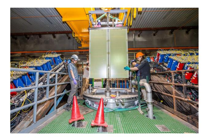
The crew moved the 2×2 prototype into place for insertion into the liquid argon cryostat, where it will collect data in the NuMI neutrino beam. Credit: Dan Svoboda, Fermilab
