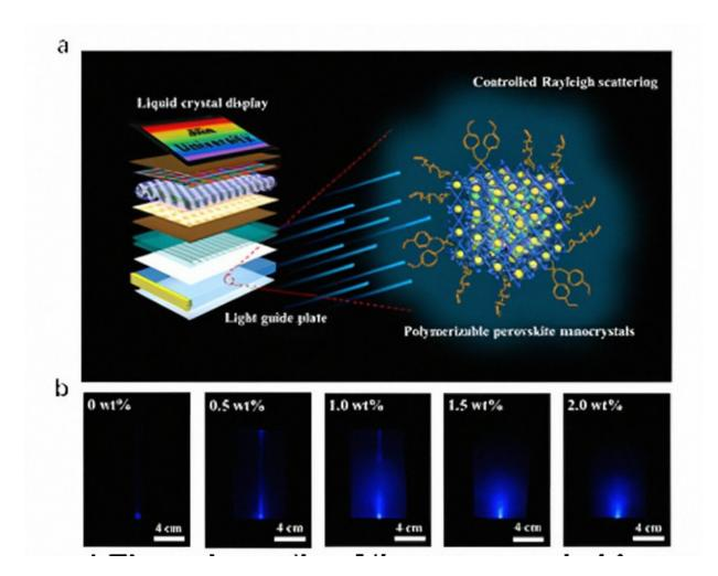
(a), The graphical abstract of the work: The PNCs/PS nanocomposite is fabricated through a two-type ligand strategy, which is proper to serve as LGP in LCD-related application based on the Rayleigh scattering behavior of the PNCs.(b), The function of LGP: When the blue laser light transports through the bulk nanocomposite with different doping content, the light and its surface output can be uniformized and enhanced. Credit: Chongming Liu, Zhicheng Zhu, Kaibo Pan, Yuan Fu, Kai Zhang and Bai Yang
