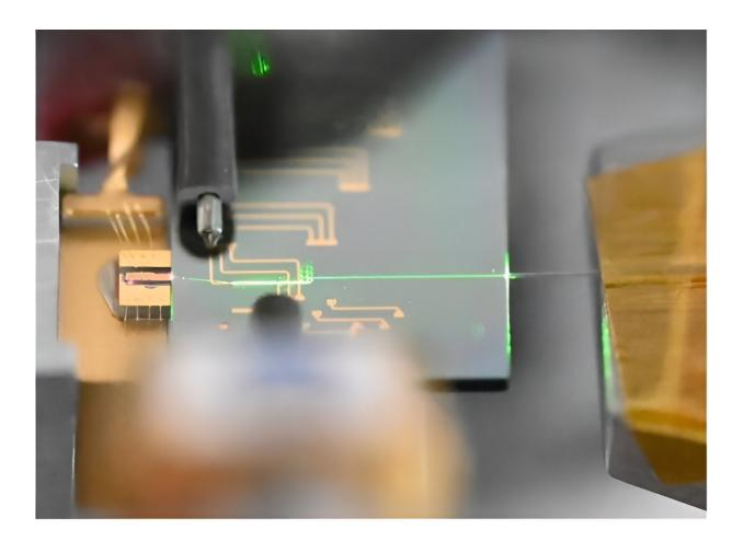
Chip scale, ultrafast mode-locked laser based on nanophotonic lithium niobate. Credit: Alireza Marandi
