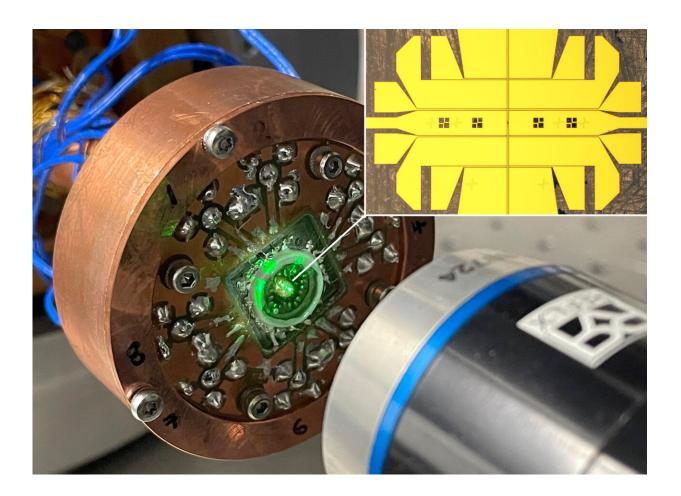
Measurement setup, in which mid-infrared and visible beams are focused onto the optoelectronic device. Insert: Image of the device on which picosecond current pulses are launched, transported and detected. Credit: Eryin Wang, MPSD
