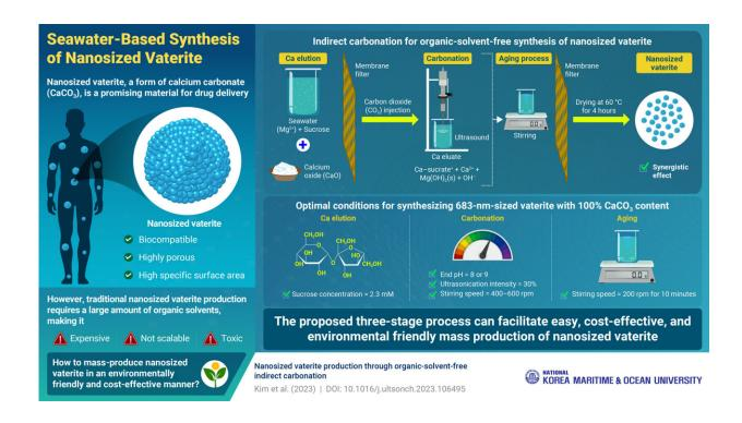
Researchers from Korea propose a three-stage process for the synthesis of nanosized vaterite that avoids the use of toxic organic solvents and produces 683-nm-sized vaterite particles with 100% calcium carbonate content. Credit: Myoung-Jin Kim, Korea Maritime & Ocean University
