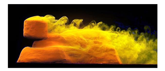
A laboratory Sphinx in the current of a water tunnel. The object is coated with clay and fluorescein dye, and the photograph captures the "streak volume" or 3D region of flow that has at some time entered the boundary layer and eroded the surface. Credit: *Physical Review Fluids* (2023). DOI: 10.1103/PhysRevFluids.8.110503
