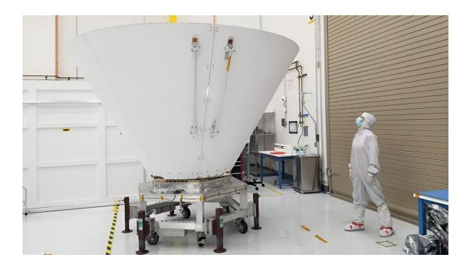
Sara Susca, deputy payload manager and payload systems engineer for NASA's SPHEREx mission, looks up at one of the spacecraft's photon shields. These concentric cones protect the telescope from light and heat from the Sun and the Earth, which can overwhelm the telescope's detectors. Credit: NASA/JPL-Caltech
