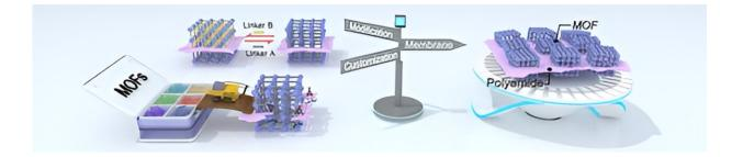
A modular customization strategy was applied for efficient MOF membrane fabrication. MOF material screening, defect-free membrane output, membrane physicochemical property regulation and separation applications can be rapidly realized by separately designing and modifying the MOF module within the membrane. High separation performance is easily achieved, which can meet diverse separation requirements. Credit: *Angewandte Chemie International Edition* (2023). DOI: 10.1002/anie.202315057
