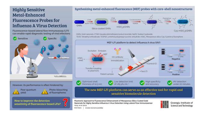
The new metal-enhanced fluorescence-based LFI platform can detect influenza A virus with great accuracy and specificity, in under 20 minutes. This technology is highly promising for biomolecule detection. Credit: Professor Min-Gon Kim, Gwangju Institute of Science and Technology
