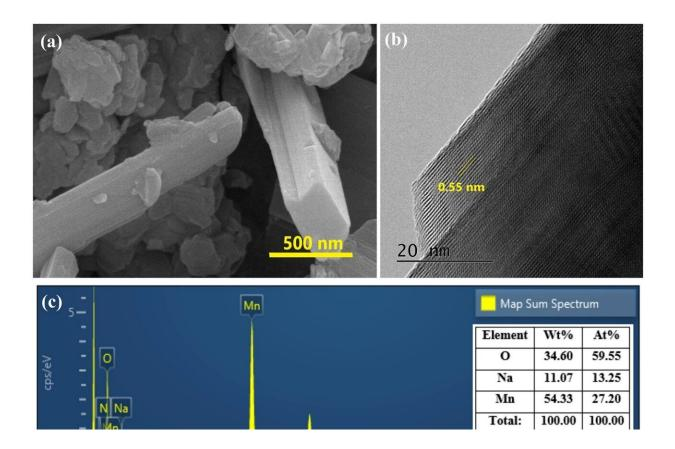
(a) SEM micrograph; (b) HR-TEM micrograph; (c) EDAX analysis; (d) 2D elemental mapping of Sodium-manganese oxide. Credit: Korea Institute of Civil Engineering and Building Technology
