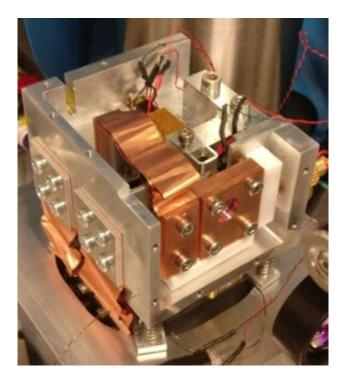
The home-built nanopositioner used to move the fiber in three dimensions over the surface if the mirror. Credit: ICFO/E. Beattie
