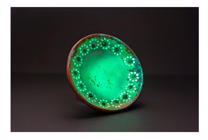
Lead detection spray on a plate. Credit: AMOLF
