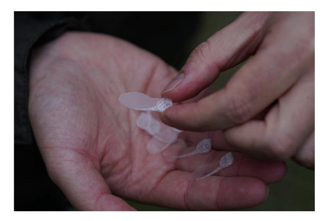
The new Acer i-Seed is made of a biocompatible and compostable material, and it has been realized with 3D printing technologies. A drone can be used to spread them out in large areas and study the terrain at a distance. Credit: IIT-Istituto Italiano di Tecnologia
