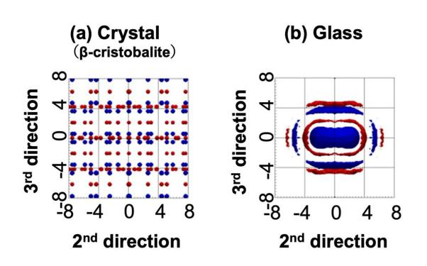
Spatial atomic densities around rings in silica crystal (left) and glass (right). Blue and red regions show large density regions of silicon and oxygen atoms, respectively. Credit: *Communications Materials* (2023). DOI: 10.1038/s43246-023-00416-w
