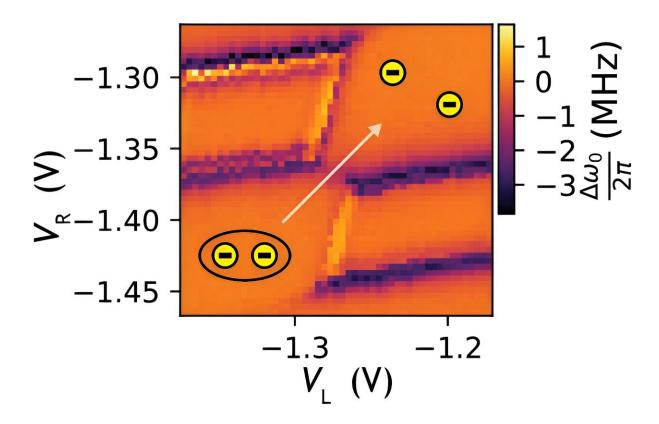
Measured shift in the resonant frequency of a microwave resonator coupled to the superconductor in our device as a function of the voltages applied to the surrounding quantum dots. The frequency shifts when electrons move back and forth between the dots and the superconductor. Moving along the line between the two diamond-like features in the diagram, a single Cooper pair is split and its
