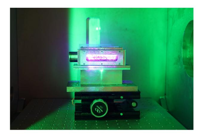
This gas cell is a key component of a compact wakefield laser accelerator developed at The University of Texas at Austin. Inside, an extremely powerful laser strikes helium gas, heats it into a plasma and creates waves that kick electrons from the gas out in a high-energy electron beam. Credit: Bjorn "Manuel" Hegelich
