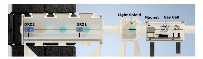
A drawing of the compact wakefield laser accelerator developed at The University of Texas at Austin. A laser beam enters on the right side and travels into the gas cell where an electron beam is created, which travels eventually to two scintillating screens (DRZ1 and DRZ2) for analysis on the left side. Credit: University of Texas at Austin
