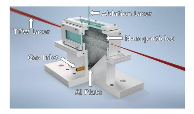
Gas cell drawing. Inside, an extremely powerful laser strikes helium gas, heats it into a plasma and creates waves that kick electrons from the gas out in a highenergy electron beam. Nanoparticles—generated by a secondary laser shining through the top window and striking a metal plate—boost the energy transferred to the electrons. Credit: University of Texas at Austin
