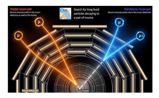
Illustration of two types of long-lived particles decaying into a pair of muons, showing how the signals of the muons can be traced back to the long-lived particle decay point using data from the tracker and muon detectors. Credit: CMS/CERN
